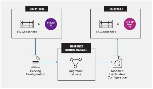
Figure 1: Process flow for BIG-IP TMOS to BIG-IP Next migrations.
